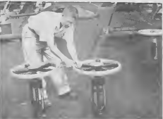
TO PREVENT mixing of different refinery products in this ship's tanks, Lt. Doyle must seal the crossover valves. PA PREVENI mezclamento di diferente productonan di rafineria den tankinan di e bapor aki, Lt. Doyle mester seya e crossover valves.
